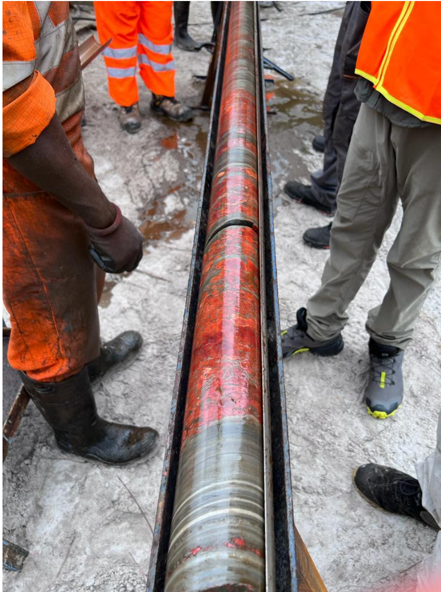
Potash-rich drill core from BA-002 Extension showing red carnallite mineralization at a depth of approx. 519m.
